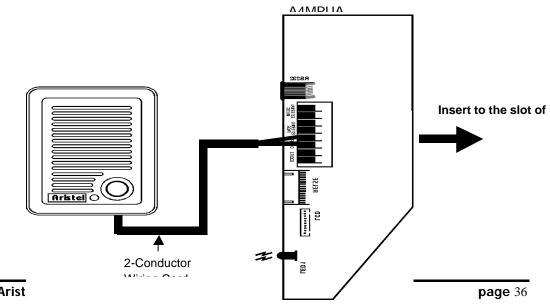
Figure 1.20 Door Phone Installation Layout
