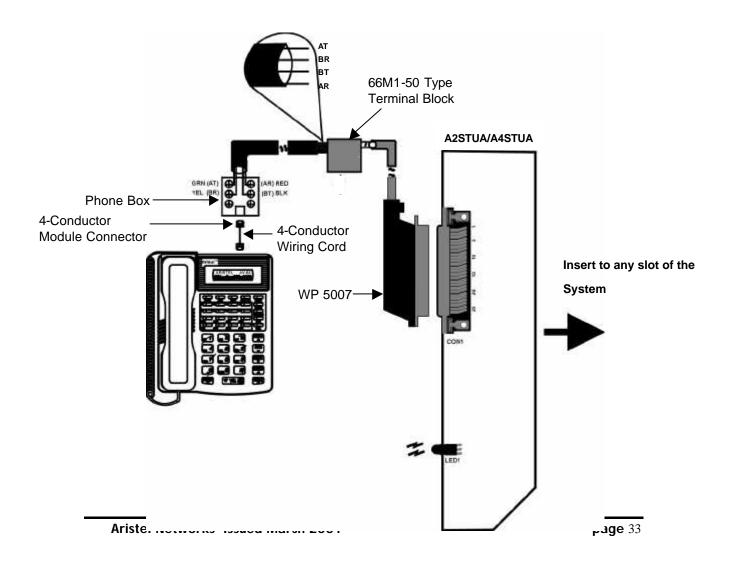
Figure 3.9 General Key Station Installation Layout
