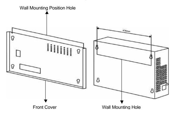
Figure 1.6 AV-256 System Wall Mount Layout
