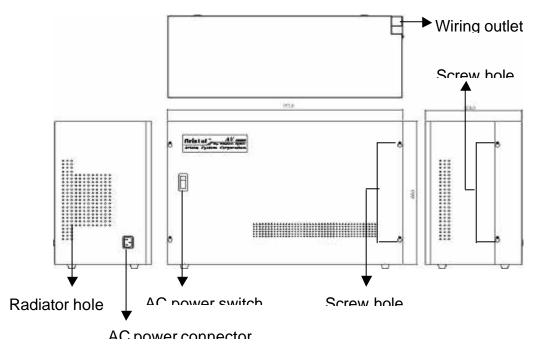
Figure 1.1 AV-256 System Three-Dimensional Layout
