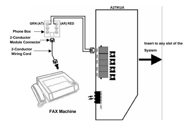
Figure 3.8 FAX Machine Installation Layout
