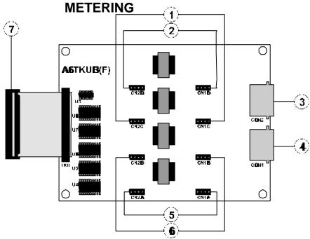
Figure 11. A6TKU4R 4 PORT TRUNK CARD WITH REVERSAL AND METERING
