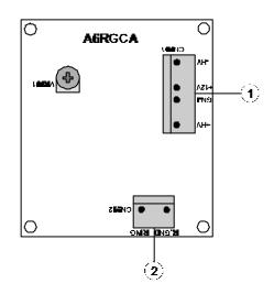
1. CN901 : 4-Wire Connector. Connect to [CN802] on the A6PWUA.
