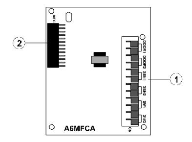
Figure 14. A6MFC Multi Function Card, 2 Sensors+2 Relays+2 Door Phones
