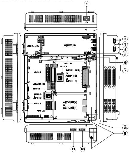
Figure 1. System Inter-Circuit Layout
