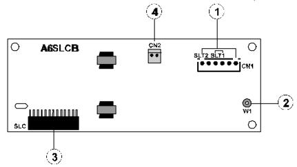
Figure 8. A6SLC 2 Port Single Line Station Card
