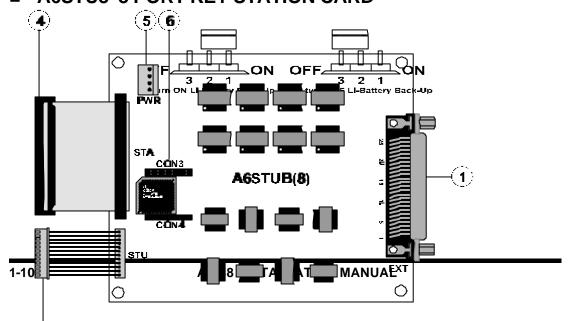
1. EXT : Amp Connector for Key Station Wiring
