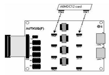
Figure 20. Metering Pulse Detection Card Installation
