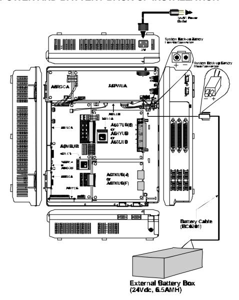
Figure 18. AC Power and DC Battery Back-Up Installation
