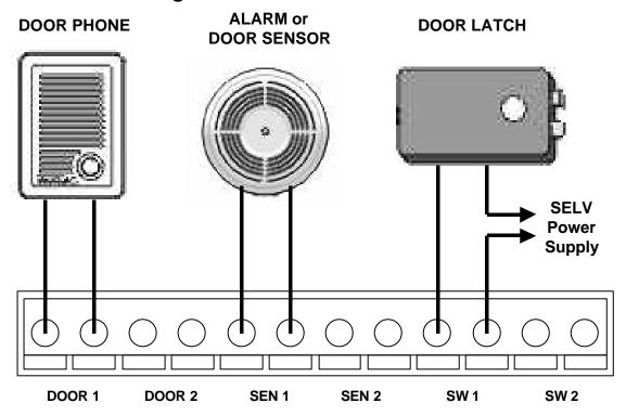
Figure 26. 2-Wire Door Phone Connection on A6MFC
