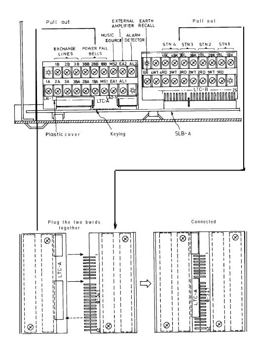
FIG. 45 - CONNECTION OF LTC-A AND LTC-B TO PROVIDE EXCHANGE LINE OPERATION WHILE CARRYING OUT SERVICE
