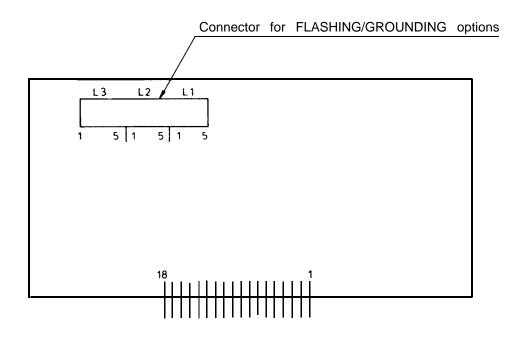
FIG. 44 - FGB-A CONNECTOR LAYOUT
