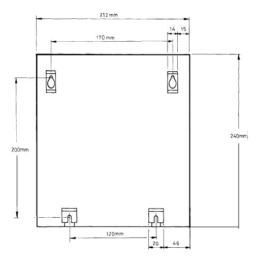
FIG. 27 -WALL MOUNTING OF POWER SUPPLY
