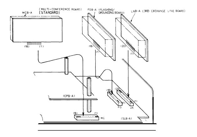
FIG. 32 - BOARD INSTALLATION (MCB-A, FGB-A, LNB-A)
