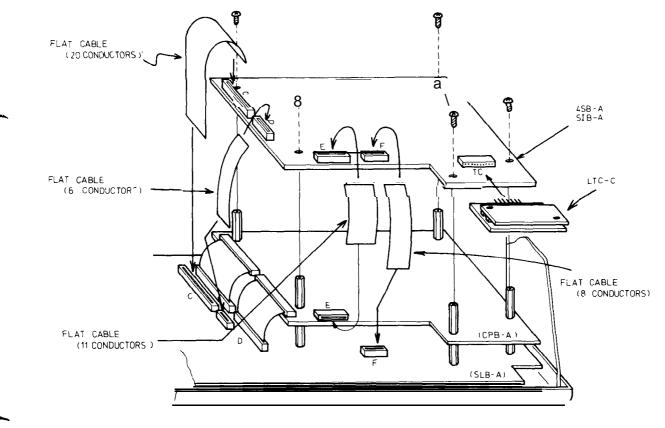
FIG. 22 - EXPANSION BOARD INSTALLATION (SIB-A, **4SB-A**)
