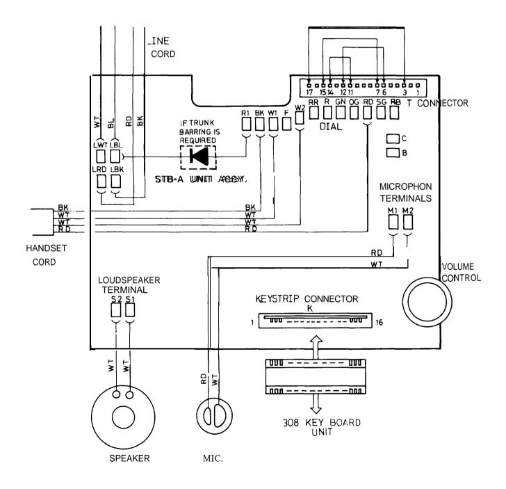
FIG. 34 - STB-A STATION BOARD ASSEMBLY
