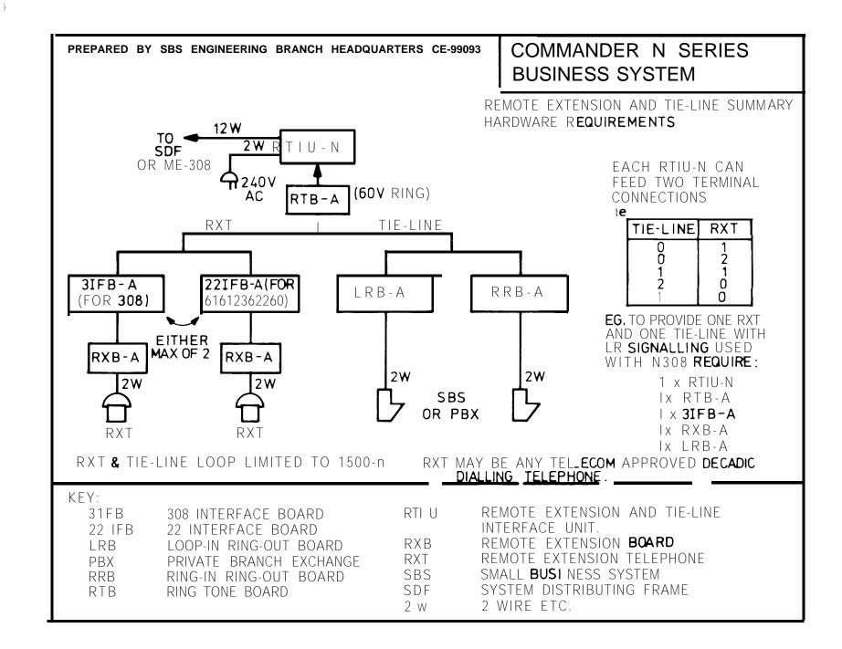
FIG. A2 - RTIU HARDWARE REQUIREMENT
