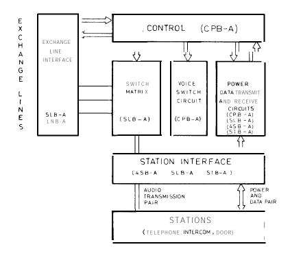
FIG. 7 - N308 MAIN EQUIPMENT BLOCK DIAGRAM
