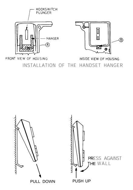
FIG. 28 - INSTALLATION OF THE HANDSET HANGER POSITIONING STATION ONTO THE WALL MOUNTING BRACKET
