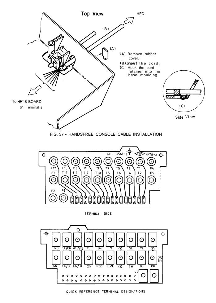
FIG. 38 - HFTB-A HANDSFREE TERMINAL BOARD
