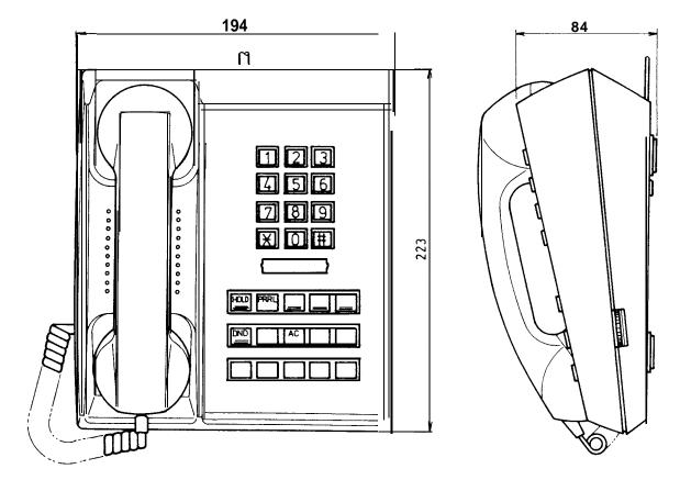
FIG. 14 - N308 TELEPHONE STATION TS-308 DEC/DEAB/VFAB
