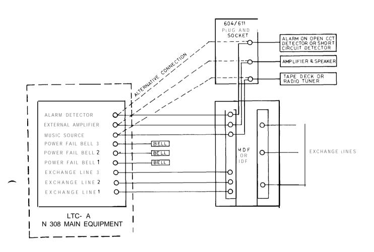
FIG. 30 - TERMINATING OF SYSTEM
