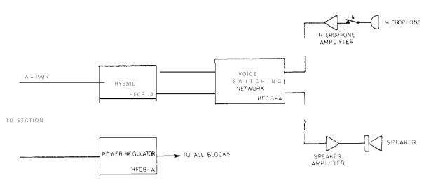
FIG. 10 - HANDSFREE CONSOLE BLOCK DIAGRAM
