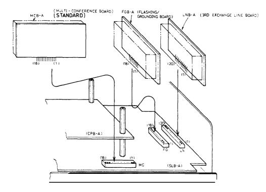
FIG. 23 - BOARD INSTALLATION (MCB-A, FGB-A, LNB-A)
