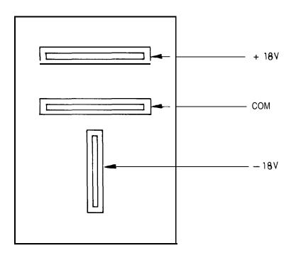
FIG. 46 - MAIN EQUIPMENT POWER SOCKET LOCATED ON SIDE OF THE POWER SUPPLY
