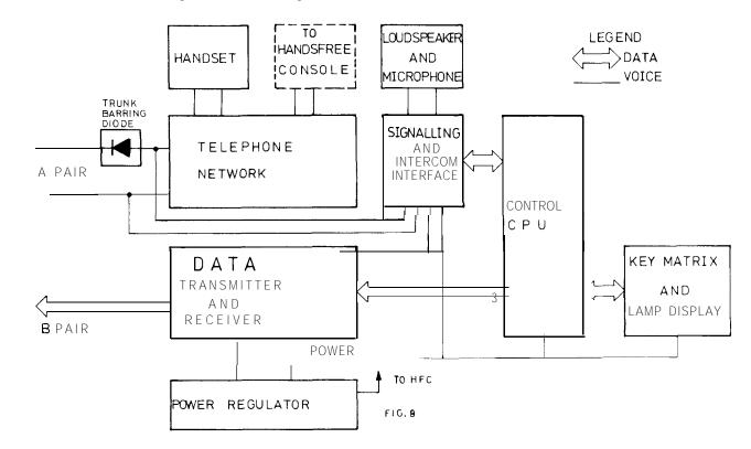
FIG. 8 - N308 TELEPHONE STATION BLOCK DIAGRAM
